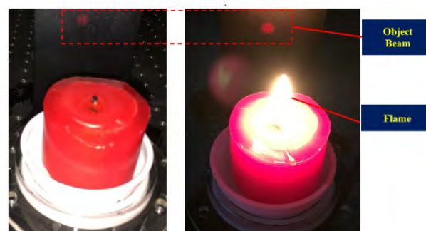
Fig. 2. Flame of Candle with Object Beam Passing through
