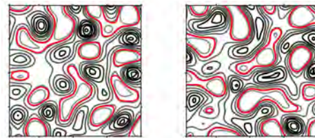
FIG. 2: Contour plots of the pattern on the lower liquid film at two consecutive timesteps with highlighted contours at a selected liquid thickness.
