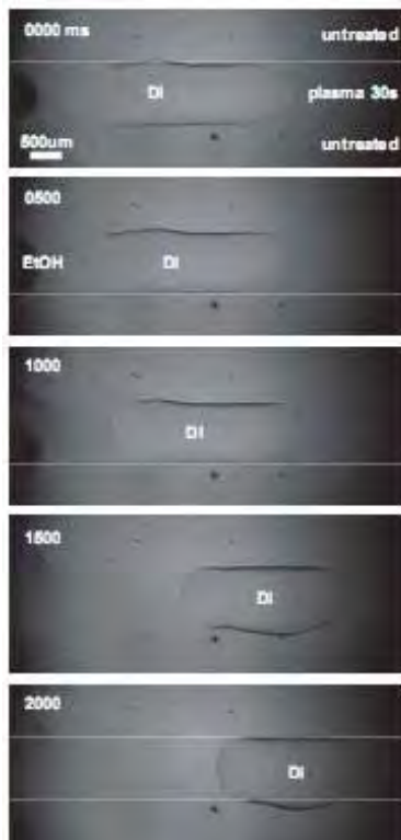
Fig. 1: Droplet actuation on a hydrophilic stripe.
